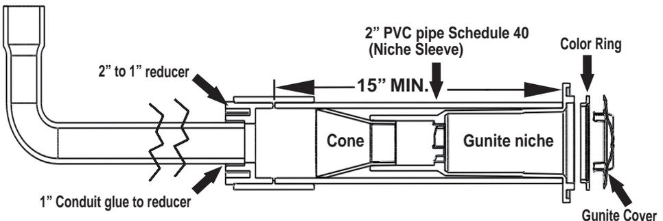
**Option 1: Niche Sleeve with Cone - Installation Diagram**
