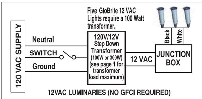
GloBrite™ LED Light with Wall Switch Wiring Diagram
